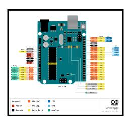
be used for both digital input and digital output. PWM is a technique used to encode a message into a pulsing signal. They are composed of 2 components: frequency and duty cycle. PWM frequency dictates how long it takes to complete a single cycle and how quickly it fluctuates from high to low. The cycle determines how long a signal stays high out of the total period. Finally, Serial, Serial communication is used to receive and transmit data between the Arduino board and another serial device.
