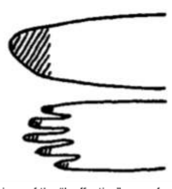
A comparison of the "ineffective" area of a wing with and without tip slotting.
